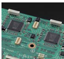
Transmit/ Receiver DSP (left) and Receiver DSP (right) ADSP-21489 by Analog Devices 32-bit floating point DSP 2400 MFLOPS 393 MHz clock speed
